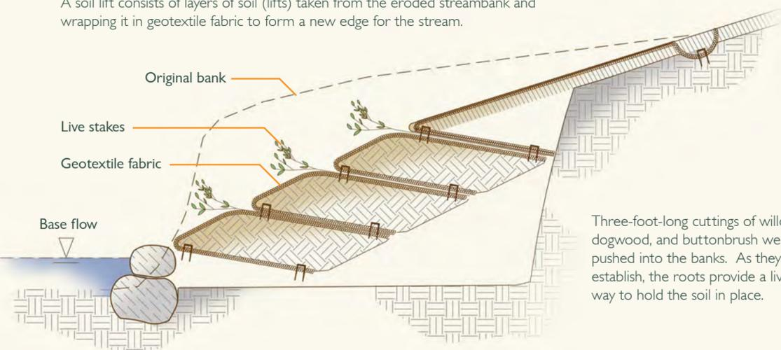
Three-foot-long cuttings of willow, dogwood, and buttonbrush were pushed into the banks. As they establish, the roots provide a living way to hold the soil in place.
