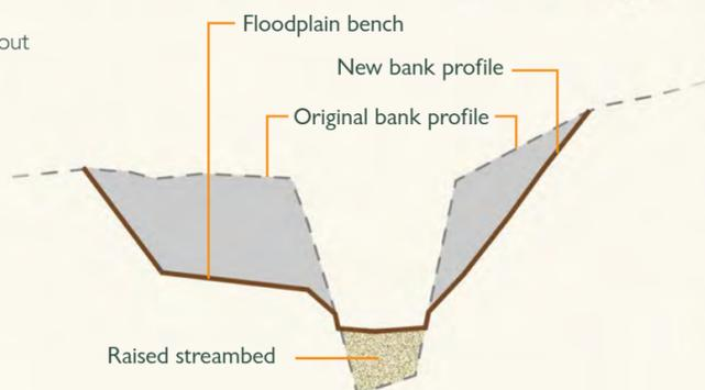
Providing floodplain connection allows the stream to leave its banks during large storm events which allows water to spread over a larger area, reducing its velocity and erosive force. It can also reduce flooding in areas downstream of the park.
