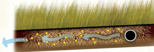
As the water flows into the buffer area, the plants and soil organisms have time to remove nutrients and other potential pollutants from the tile before it reaches the stream.
