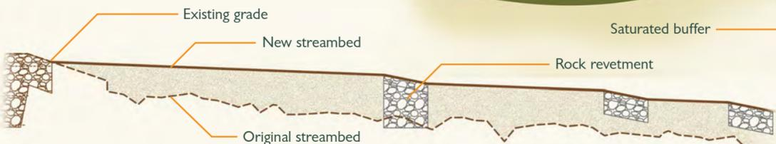
The stream was reconnected to the floodplain throughout the corridor by raising the streambed or by excavating floodplain benches adjacent to the channel.
